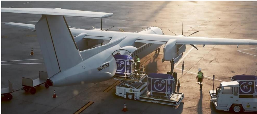
Figure 7: Universal Hydrogen illustration of proposed Dash-8 Aircraft hydrogen conversion using gaseous hydrogen capsules. Credit: Universal Hydrogen.
