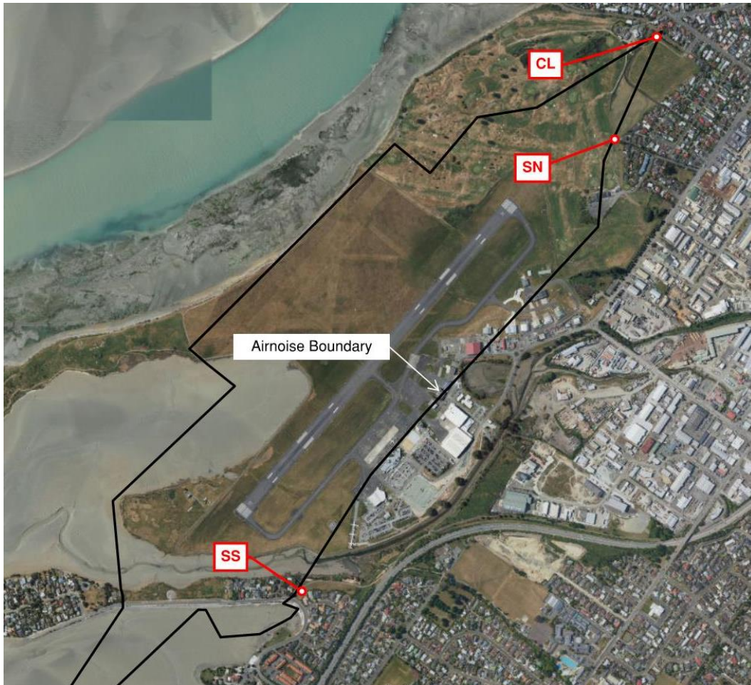
Figure 1: Current noise monitoring locations CL, SN and SS on the Airnoise Boundary
